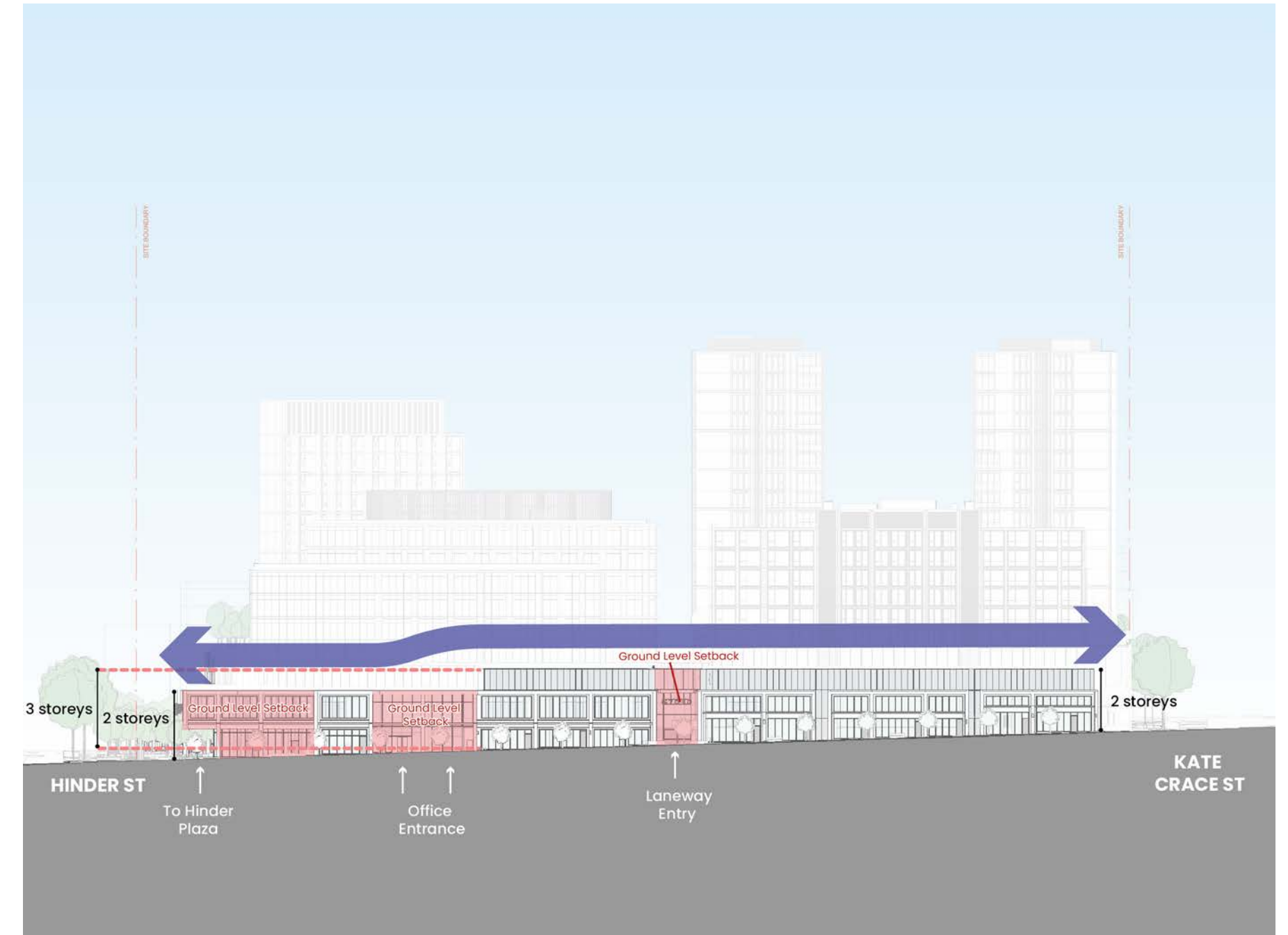
Figure 11 Hibberson Street elevation, with annotations emphasising the podium streetwall (Source: COX, with annotations)
